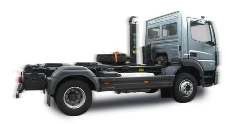
Body with hook height 1425 mm Welded hook
