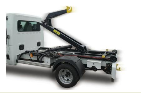
Tilting hook arm for lower lifting angle
